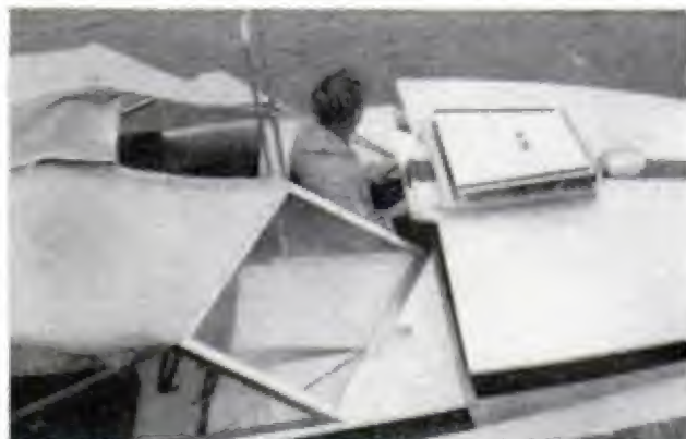
THOUGH FOREDECK LOOKS HEAVY , 5-ft.-long section is easily lifted if firmly gripped in the middle
